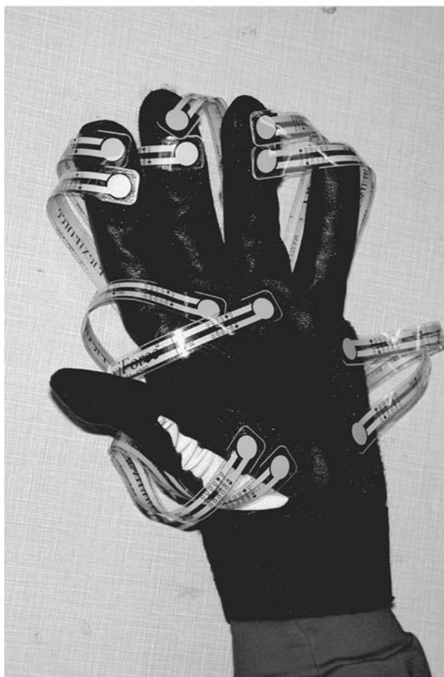
Fig. 2 (A) Photo of the sporting glove fitted with 444 N-range Flexiforce pressure sensors (Tekscan Inc., South Boston, MA, USA) used to quantify the forces applied to subjects during the Push and Release Test and the Pull Test.
