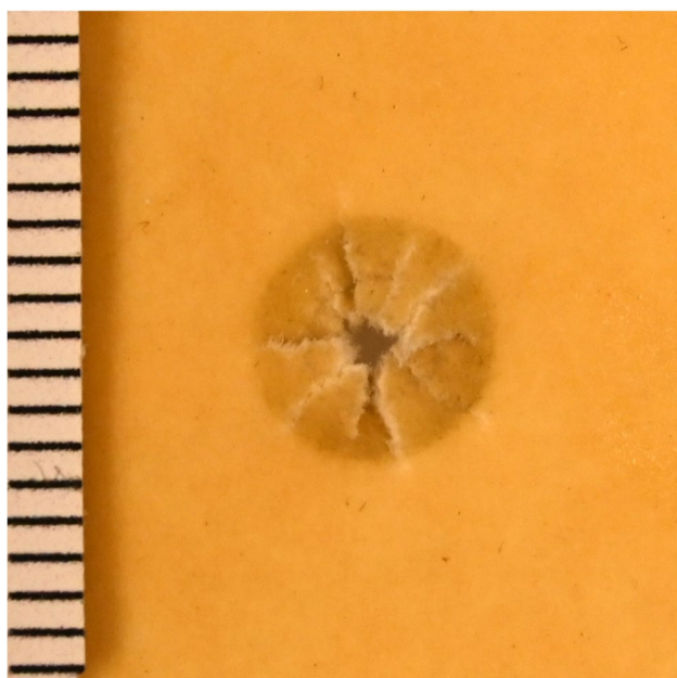
Fig. 4 Dental silicone shore hardness 22-chamois leather-compound (perpendicular shot, 10 m distance)
