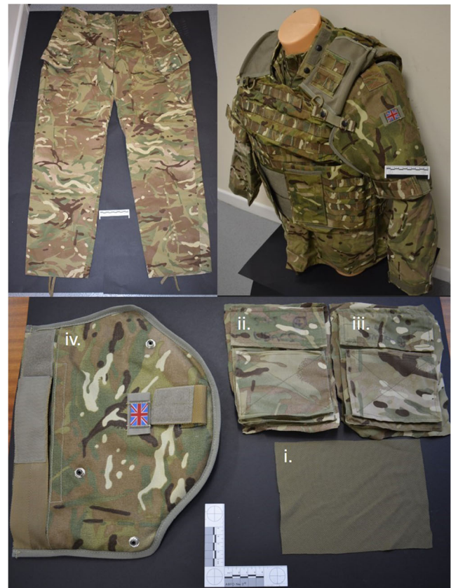
Fig. 1 Examples of MTP clothing used—clockwise from top left: MTP trousers; top right: t-shirt, UBACS, smock and brassard as worn by service personnel; bottom: i. t-shirt, ii. UBACS, iii. smock and iv. brassard layers prepared for testing. Laundering detail and fabric analysis data for this clothing used within these experiments is detailed in previously published work [29]
