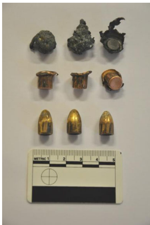
Fig. 4 Typical examples of recovered bullets, jackets and cores ( top row Remington R357M3 cores, middle row Remington R357M3 jackets, bottom row 9 mm FMJ)
