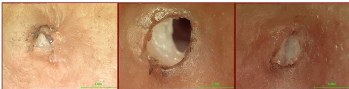
Fig. 15 Typical wounds created by Phillips screwdrivers in pork leg
