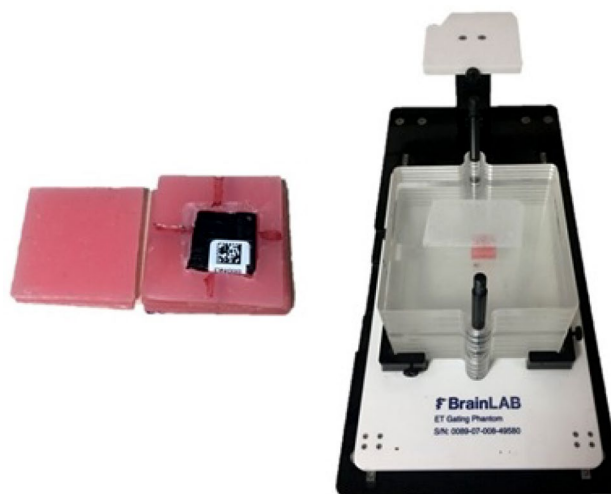
Fig. 1 Optically Stimulated Luminescence (OSL) dosimeter inside the paraffin material used to simulate a tumour, and the phantom setup used for imaging and irradiations
