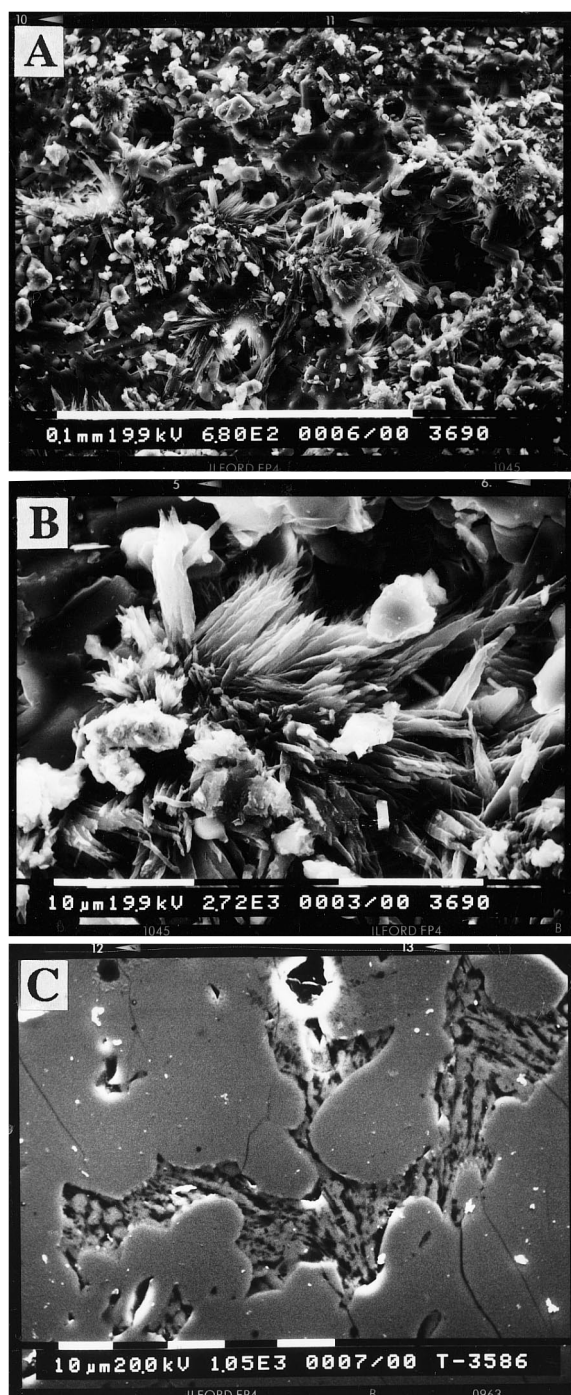
Fig. 2A–C Back scattered electron images of A unpolished material from run T-3690 (71001), showing abundant spheroidal cavities indicative of the presence of a free fluid phase. In addition, needles of quenched (Na,Mg)-carbonate are visible. B Closer view of quenched carbonatite in T-3690. Needles are (Na,Mg)-carbonate. Small euhedral white grains are dolomite. C Carbonatite melt trapped in annealed layer of coarse San Carlos olivine grains which were included in T-3586. Quench structures are clearly visible
