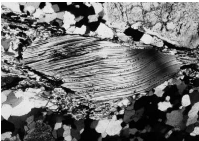
Fig. 1 Photomicrograph of porphyroblast of muscovite sheared along the basal plane under greenschist facies conditions (sample 796 of Dunlap 1997), long dimension \sim 1.5 mm. Deformation of the porphyroblast is predominantly by dislocation glide within the cleavage plane, resulting in the undulatory extinction, but there is some evidence for the operation of additional deformation mechanisms, including kinking and cracking (resulting in the finer grains that appear to be torn away from the porphyroblast), and possibly cataclasis and chemical alteration between cleavages (resulting in the darker amorphous zones). Neocrystallized mica has also formed in the fine grained groundmass (Dunlap 1997)
