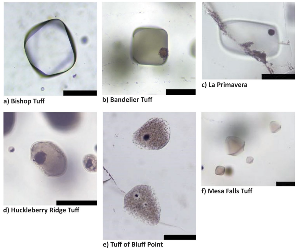
Fig. 1 Photomicrographs of target melt inclusions in quartz crystals from the eruptions listed in Table 1. All scale bars are 100 \mu\text{m} . For samples with cracks (Bluff Point and Primavera), the cracks were found to be fully contained within the crystal before sample preparation began. The Bandelier, La Primavera, Huckleberry, and Bluff Point inclusions contain volumetrically small bubbles (< few vol.%). Bishop and La Primavera inclusions are clear glass whereas Huckleberry and Bluff Point inclusions are brown and contain incipient crystals. All inclusions are partially or fully faceted. The dark smudge on the lower side of the Primavera inclusion is polishing paste
