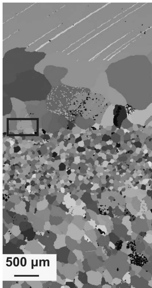
Fig. 2 EBSD map of the central part of the sample. Greyscales correspond to different grain orientations. Patterns were collected automatically at 10 \mu\text{m} intervals and processed using Channel ® software. Note the twinned single crystal at the top of the image, the recrystallized zone adjacent to the fine powder layer, and Carrara marble with a weak grain shape fabric at the bottom. The box indicates the area of Fig. 3. The area of Fig. 4 extends beyond the left-hand edge of the EBSD map
