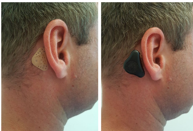
Fig. 1 The ADHEAR system with its adhesive adapter (left) and the audio processor (right)
