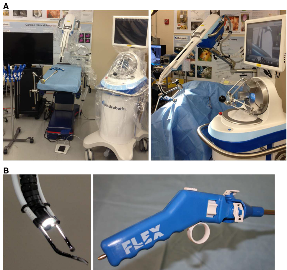
Fig. 1 a Medrobotics Flex ® System. The system consists of five components: the Flex Console which houses the surgeons control handle and a touch screen visual display and the touch screen monitor; the Flex Base, a reusable assembly that translates electronic signals from the console into mechanical motions; the Flex Scope, a sterile, disposable for transfer of mechanical motions from the base to the endoscope; the table mounted stand as support for the base and disposable and the Flex Cart. b Photograph of the distal tip of the flexible endoscope system with the HD camera, LED lamps and flexible 3.5-mm instruments inserted through the two accessory channels, and of flexible instrument control for 3.5-mm flexible instruments with distal wristed end-effectors
