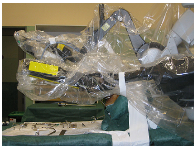
Fig. 1 The cadaver head placed on the platform, on the operating table, fixed with tape. The da Vinci system was placed cranially in order to give the robotic arms greater maneuverability while the terminals and endoscope were directed at the soft palate and rhinopharynx
