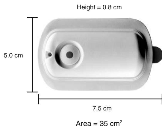
Fig. 1 The fentanyl HCl iontophoretic transdermal system (fentanyl ITS). Figure is reproduced with permission [6]
