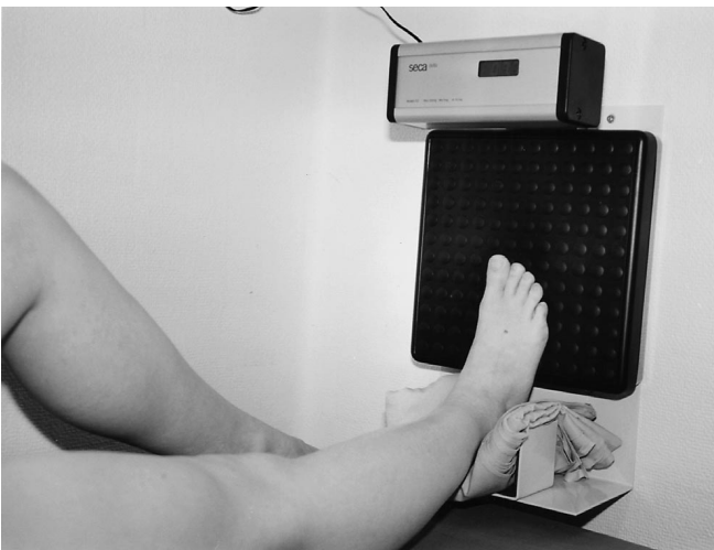
Fig. 2 Self-constructed instrument to measure the ankle-power in kilograms, while the patient is lying on a stretcher pushing against the scale
