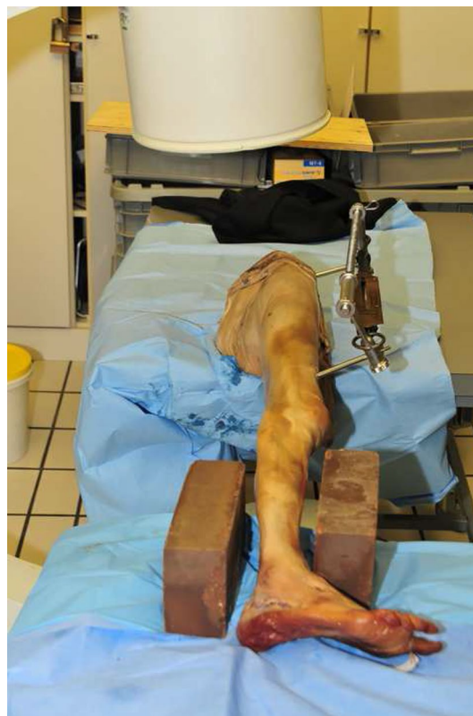
Fig. 1 Laboratory set-up with mounted large femoral distractor to apply traction under radiographic control
