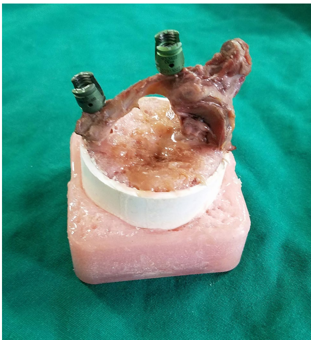
Fig. 3 Atlas vertebra with PS or PAS was embedded in custom-made molds using polymethylmethacrylate cement
