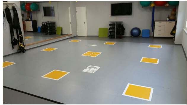
Fig. 1 SpeedCourt-interactive training device, consisted with an active area for 7 × 7 m and 15 integrated and coded measure plates
