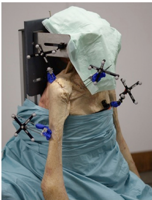
Fig. 1 Experimental setup with sitting body in the special and fixation. Four marker of the optic navigation system (Polaris P4, NDI, Waterloo, Canada) (sternum, clavicle, acromion and humerus)
