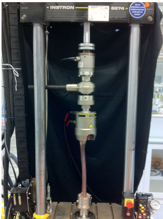
Fig. 4 The testing mechanism. The composite femur and stem are fitted in the Instron. Reprinted from Morishima et al. [18]. Copyright (2014), with permission from Elsevier
