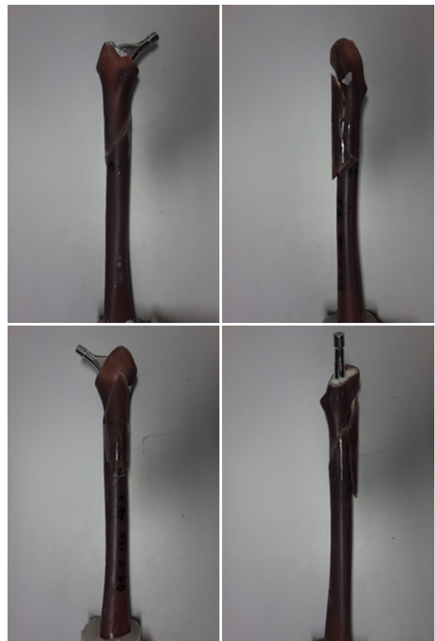
Fig. 5 Example of the fracture pattern of an Exeter 44-4 stem created by our testing mechanism
