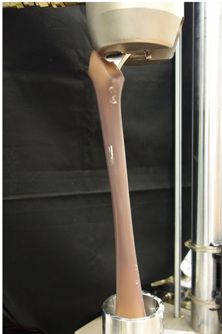
Fig. 3 The femoral head and intercondylar notch are located in the vertical loading axis of the machine to replicate the natural loading axis of the femur. The proximal femur is attached at the centre of rotation of the implant head by means of a hydraulic clamp. Reprinted from Morishima et al. [18]. Copyright (2014), with permission from Elsevier
