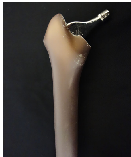
Fig. 2 Example of how a stem is fitted in the composite sawbone. The three markings on the stem can be used to determine the position of the stem. Reprinted from Morishima et al. [18]. Copyright (2014), with permission from Elsevier
