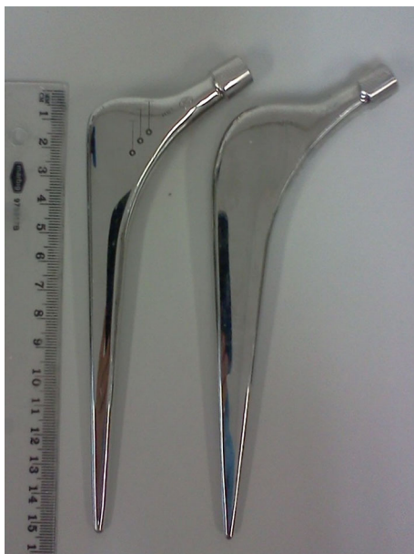
Fig. 1 The left stem shown is an Exeter 44-1 stem, and the right stem shown is the 44-4. Notice the increased body size
