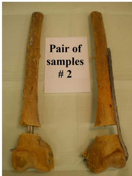
Fig. 1 A typical postoperative anterior–posterior photograph showing anatomic reduction and stabilization using a reamed retrograde femoral nail ( right femur ) and a non-contact bridging plate ( left femur )
