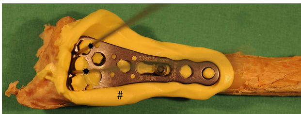
Fig. 3 Palmar view of the left dorsal radius as in Fig. 2 with K-wire (asterisk)-fixed Königsee plate 5/3 holes impressed into Optosil Comfort Putty (hash)
