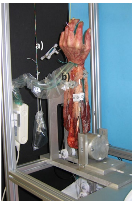
Fig. 2 Biomechanical test-setup with the specimen in extension. Range of motion was recorded by an ultrasound-based system (a). The intraarticular sensor was inserted dorsally into the radiocarpal joint (b)
