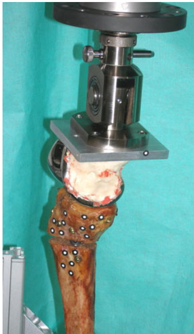
Fig. 3 Testing sample with markers for displacement measurement and compensator to achieve physiological load sharing
