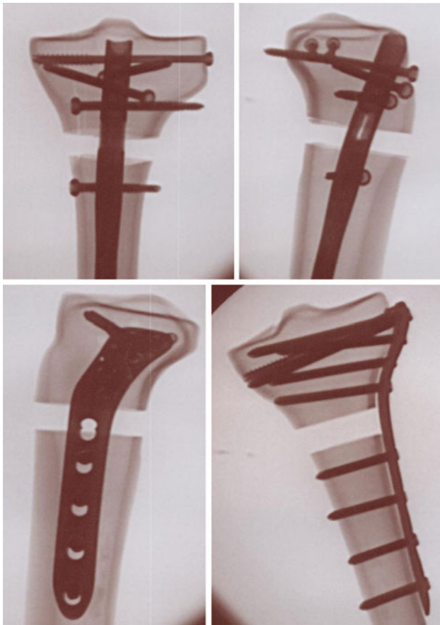
Fig. 2 X-ray after instrumentation with lag screw, nail or plate before biomechanical testing
