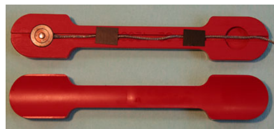
Fig. 2 Feeler gauge with integrated force probe
