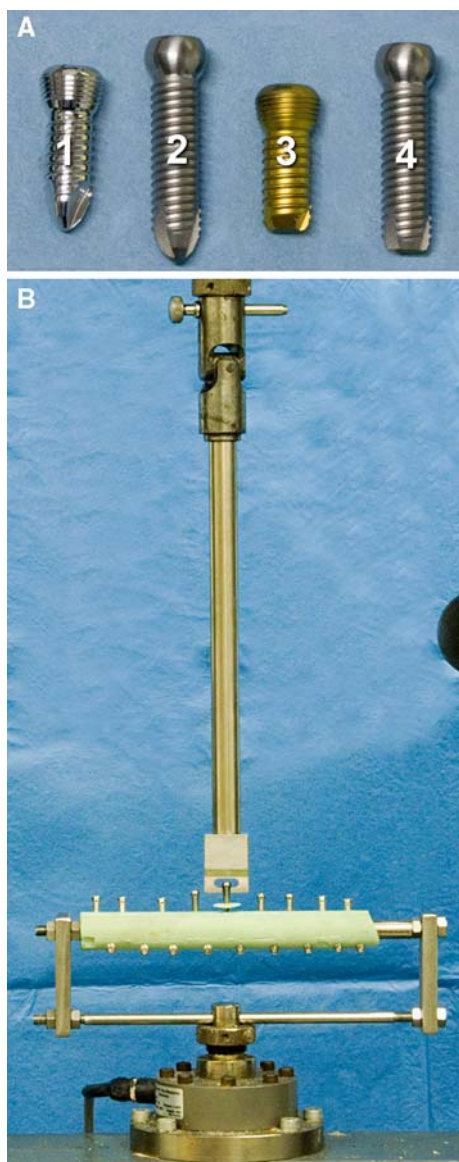
Fig. 2 a The four different tested screws; locking head screw: LHS (1), NCB screw: NCB (2), periprosthetic locking screw: PPLS (3) and periprosthetic NCB screw: ppNCB (4). b Setting for the pullout test of a unicortical screw
