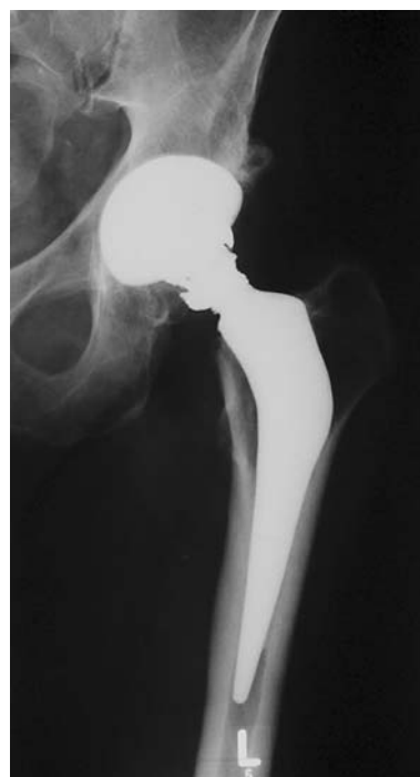
Fig. 2 Anatomical adapted stem and a cementless cup with a ceramic inlay. Typical signs of debris around the neck after fracture of the ceramic head
