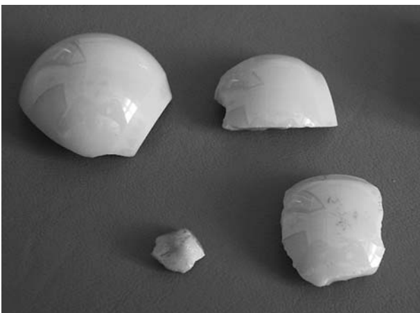
Fig. 6 Fractured ceramic head
