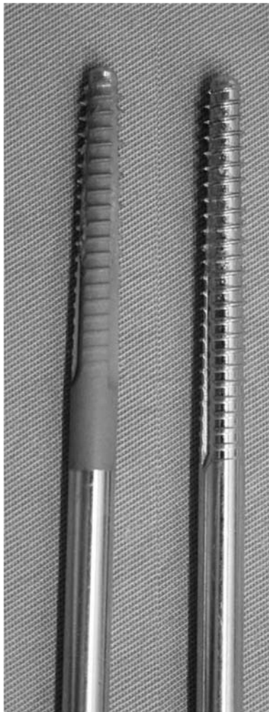
Fig. 1 Hydroxyapatite-coated Schanz screw ( left ) and standard stainless steel screw
