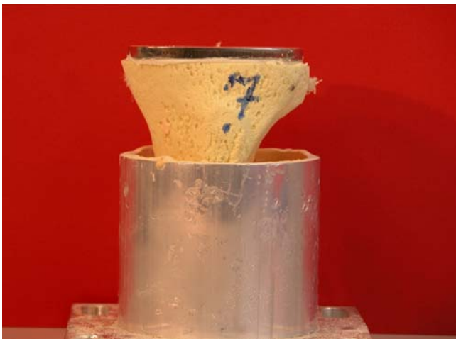
Fig. 1 Tibial tray cemented in sawbone model with 3 mm cement under the tibial baseplate fixed in the holding device for Zwick's machine
