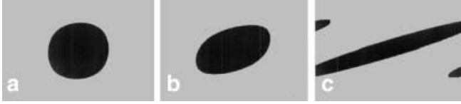
Fig. 2a–c Deformation of a 2D droplet with diameter 750 nm subject to shear flow with a shear rate of: a \dot{\gamma} = 0.01 \text{ s}^{-1} ; b \dot{\gamma} = 0.1 \text{ s}^{-1} at shear strain \gamma=3 (corresponding to steady state). Neglecting hydrodynamic interaction ( c ) the droplet is highly deformed even with small shear rate \dot{\gamma} = 0.01 \text{ s}^{-1} (deformation has still not reached its steady state at strain \gamma=3 which is shown in c )
