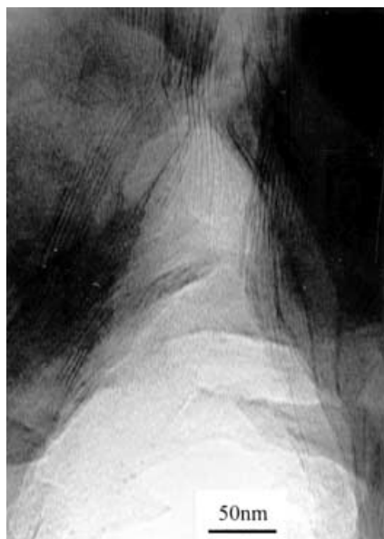
Fig. 4 High-resolution electron microscopy images of PU/OMT nanocomposites (sample a2)
