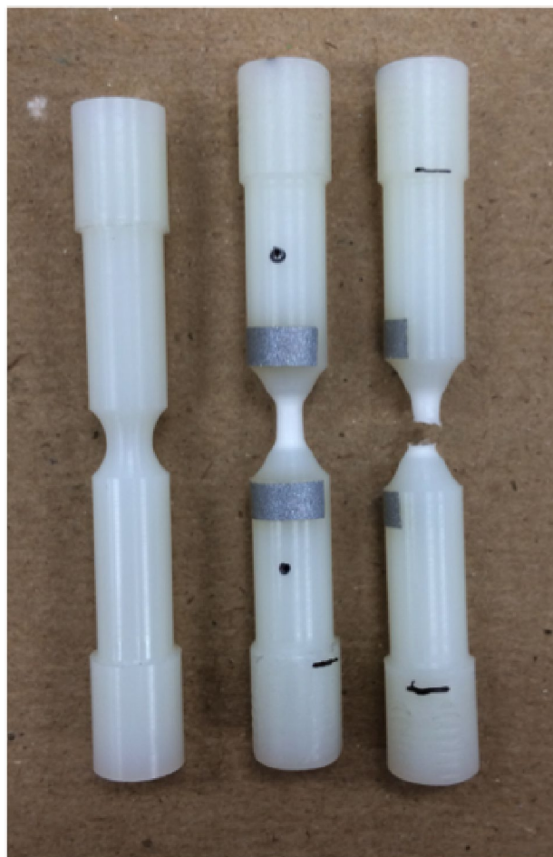
Fig. 10 An undeformed PA-6 RN10 bar (left). A PA-6 RN10 bar loaded past the peak nominal stress after storage for 217 days with a desiccant ( \text{CaSO}_4 ) (center). A PA-6 RN10 bar loaded to fracture after storage for 217 days with a desiccant (right). After absorbing ambient moisture during storage, the material was ductile enough that the notches in the specimen became locally cylindrical during loading
