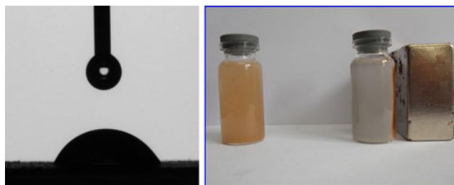
Fig. 7 The profile of water contact angle of MMIPs (left); the photograph of the dispersion of MMIPs in the absence and in the presence of an external magnetic field (right)
