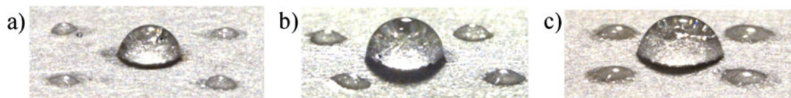
Fig. 11 Images of multiple dot designs fabricated with carnauba wax and a unmodified, b pressed with 320 grit sandpaper, and c pressed with 600 grit sandpaper
