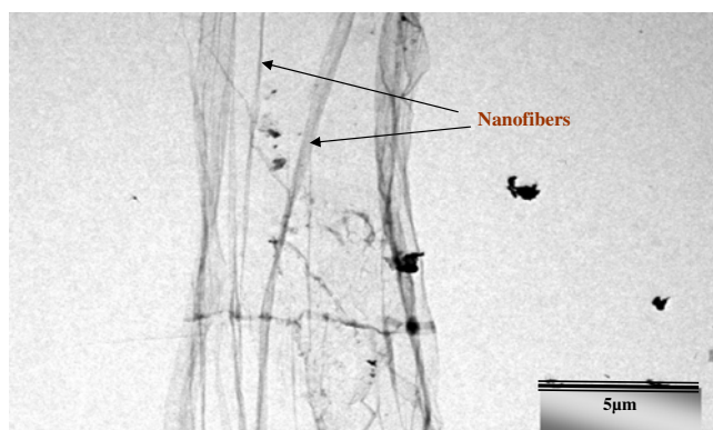
Fig. 2 TEM image of polyaniline nanofibers
