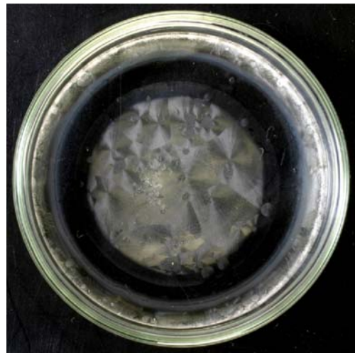
Fig. 8 Drying dissipative patterns of aqueous NaPMA solutions in a glass dish at 24 ^{\circ}\text{C} ; 0.02 monoM, 4 ml, after 54 h 25 m
