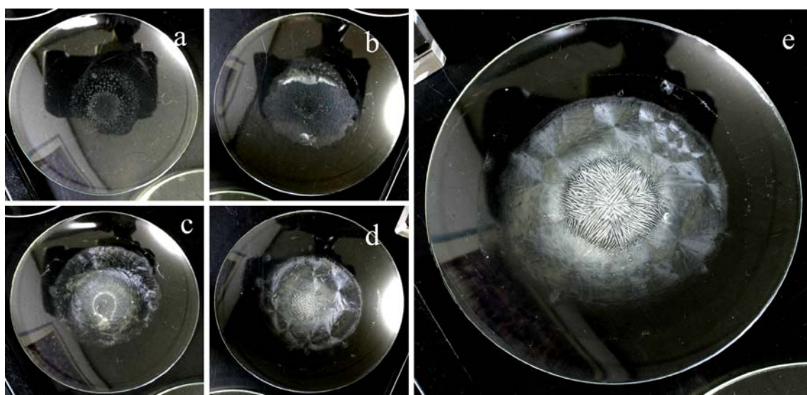
Fig. 6 Drying dissipative patterns of aqueous NaPMA solutions in a watch glass at 24 °C; 4 ml, after 54 h 25 m, a 0.000333 monoM, b 0.001 monoM, c 0.00333 monoM, d 0.01 monoM, and e 0.02 monoM
