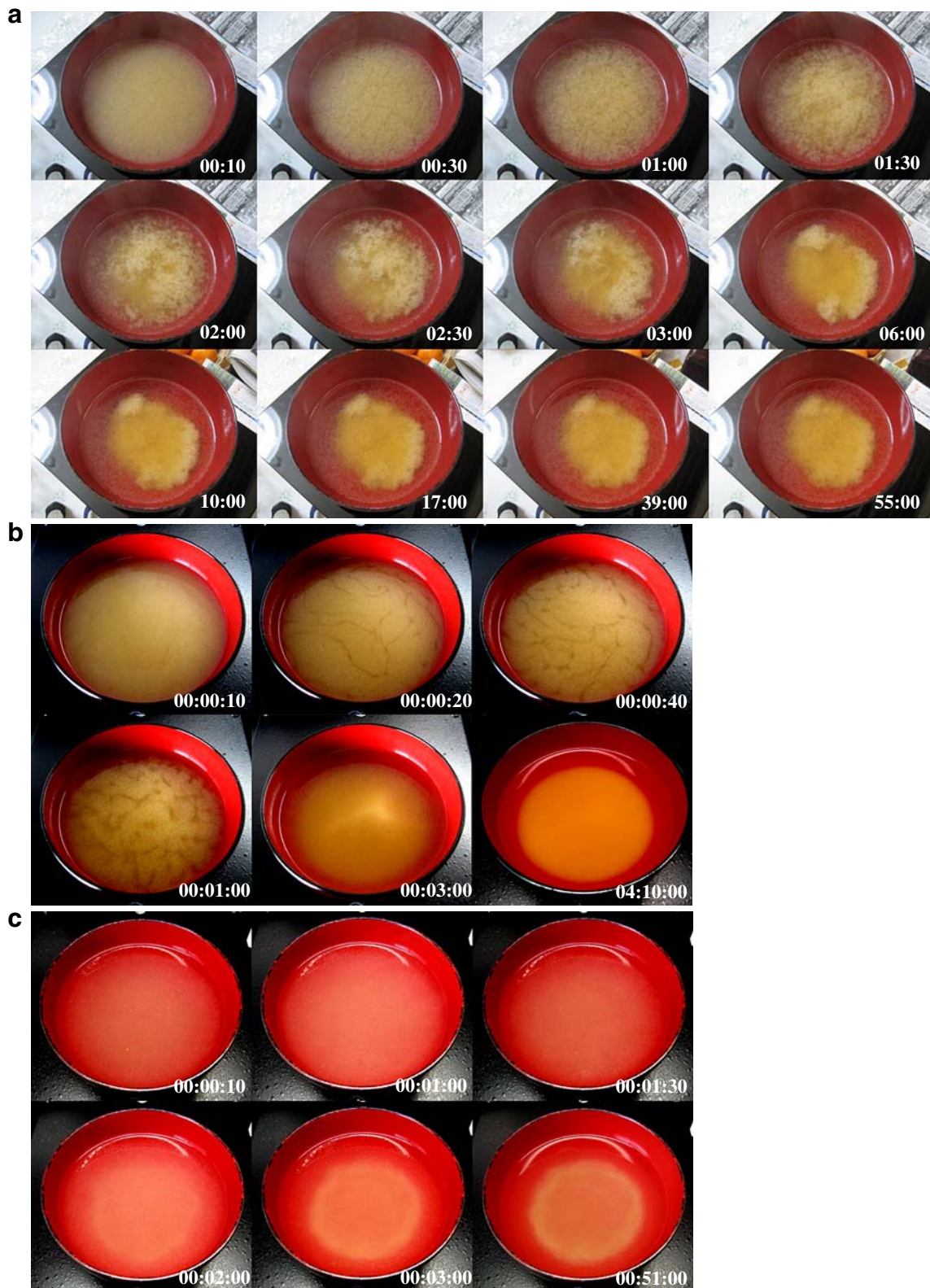
Fig. 2 a Convectonal patterns of type I Miso soup in a bowl from approximately 50 °C to 25 °C. Experiment 8, time (minutes:seconds). Miso I=0.06 g/ml, 180 ml. b Convectonal patterns of type II Miso soup in a bowl from approximately 60 °C to 30 °C. Experiment 3,
