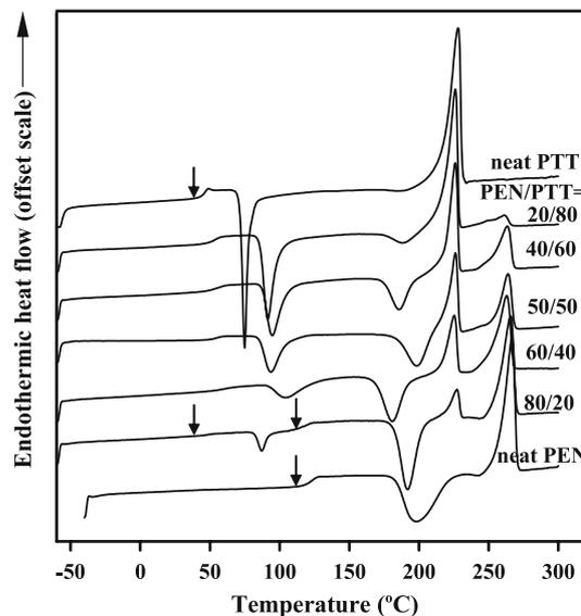
**Fig. 1** DSC thermograms (20°C/min) for PEN/PTT blends (solvent coprecipitated) and two neat polymers (PEN and PTT)
