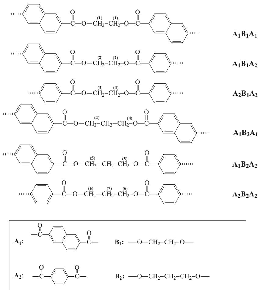
block is the original ethylene naphthalate unit, while A<sub>1</sub>B<sub>1</sub>A<sub>2</sub> represents one of the exchanged blocks where the terephthalate of PTT has been exchanged with PEN.
