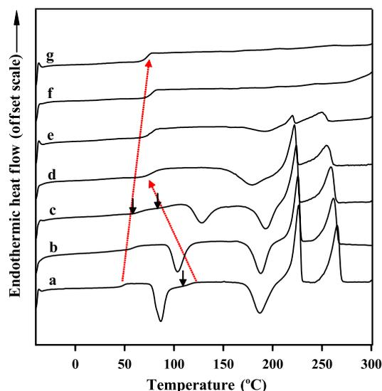
**Fig. 8** DSC traces of coprecipitated ternary EN-co-TT/PEN/PTT blends of different compositions: **a** 0/50/50, **b** 10/45/45, **c** 30/35/35, **d** 50/25/25, **e** 70/15/15, **f** 90/5/5, and **g** 100/0/0 (weight ratios)
