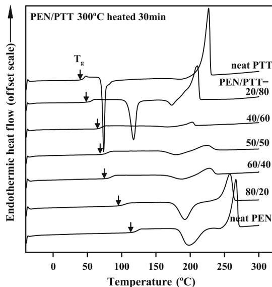
**Fig. 3** DSC traces of coprecipitated PEN/PTT blends of different compositions (weight ratio) after heating at 300°C for 30 min
