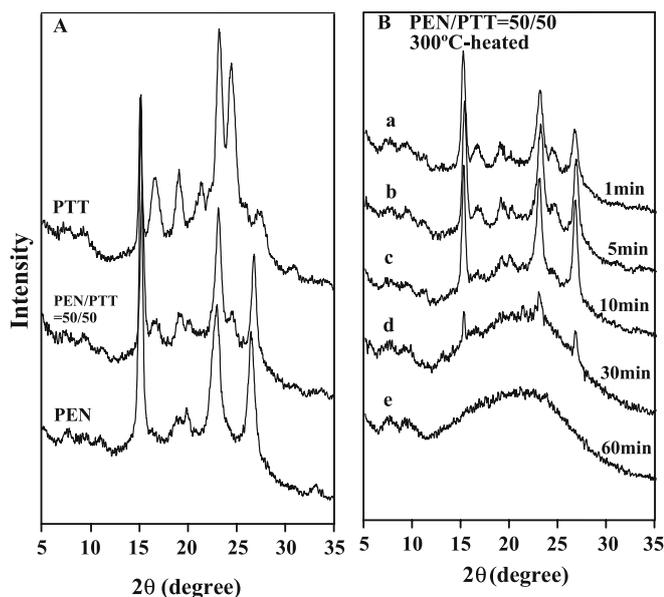
**Fig. 5** X-ray diffraction patterns of coprecipitated PEN/PTT=50/50 melt crystallized at 200°C for 8 h. **a** Without reaction and **b** after heating at 300°C for different times: (a) 1, (b) 5, (c) 10, (d) 30, and (e) 60 min
