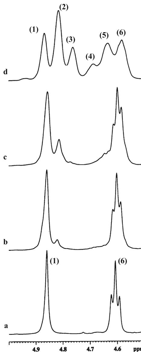
**Fig. 6**  $^1\text{H}$  NMR spectra of coprecipitation PEN/PTT=50/50 after heating at 300°C for different times: **a** 0, **b** 60, **c** 120, and **d** 480 min
