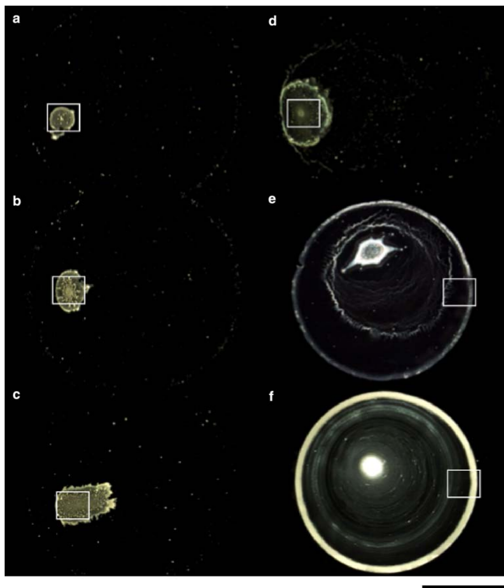
Fig. 3 Patterns formed for PEG2000000 at 25 °C. a [PEG2000000] = 1 \times 10^{-7} monoM, b 1 \times 10^{-6} monoM, c 1 \times 10^{-5} monoM, d 1 \times 10^{-4} monoM, e 1 \times 10^{-3} monoM, f 0.01 monoM. In water, 0.1 mL, length of the bar is 4.0 mm. Extended pictures of the area given by squares are shown in Fig. 4
