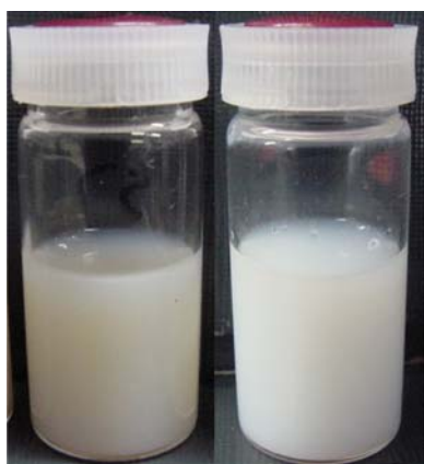
Fig. 1 Photographs of the polystyrene colloid obtained by enzyme-mediated (run 9) emulsion polymerization (left) and that by KPS-initiating emulsion polymerization (right)
