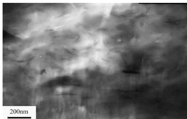
Fig. 2 Transmission electron microscope (TEM) image of a nanocomposite based on PA6 filled with 5 wt% OMT (PA6/OMT)
