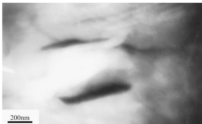
Fig. 4 TEM image of a microcomposite based on PA6 filled with 5 wt% MMT (PA6/MMT)
