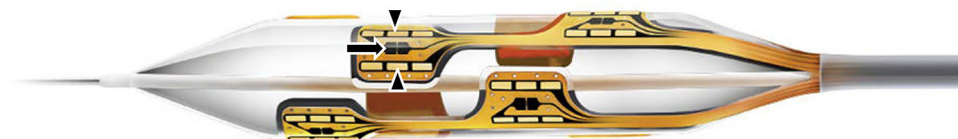
Fig. 2 Illustration of the helical array of bipolar electrodes (electrode pair indicated with arrowheads ) and thermistors ( arrow ) mounted on the Vessix balloon catheter. Used with permission of Boston
