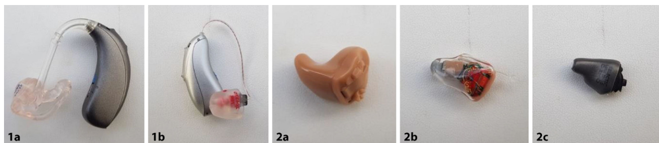
Fig. 1 ▲ Different designs of hearing aids. 1a behind the ear (BTE), 1b BTE with receiver in the canal (RIC), 2a in the canal (ITE), 2b completely in the canal (CIC), 2c invisible in the canal (IIC)
