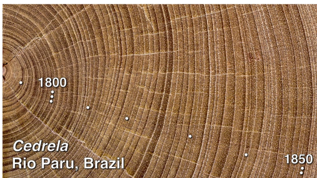
Fig. 4 This polished cross-section illustrates the clear annual growth rings on a Cedrela sp. cross-section cut during a legal operation near the Rio Paru (this portion of the specimen dates from 1785 (pith) to 1856, decades noted with white marks). The annual growth rings of this species are readily distinguished by semi-ring porosity and marginal parenchyma. The micro ring at 1833 is locally absent and difficult to see in this image
