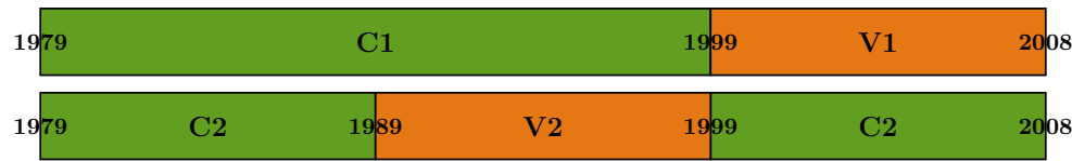
Fig. 2 Cross-validation scheme over the period 1979–2008 with two calibrations ( C_1 = [1979–1998] and C_2 = [1979–1988] \cup [1999–2008] ) and two validations ( V_1 = [1999–2008] and V_2 = [1989–1998] )
