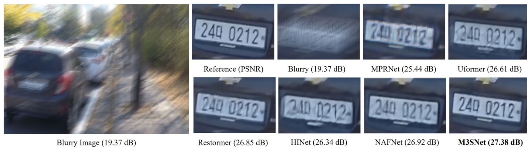
Fig. 6 Image deblurring example on the GoPro dataset [67]. Compared to the state-of-the-art methods, our M3SNet restores sharper and perceptually-faithful images
