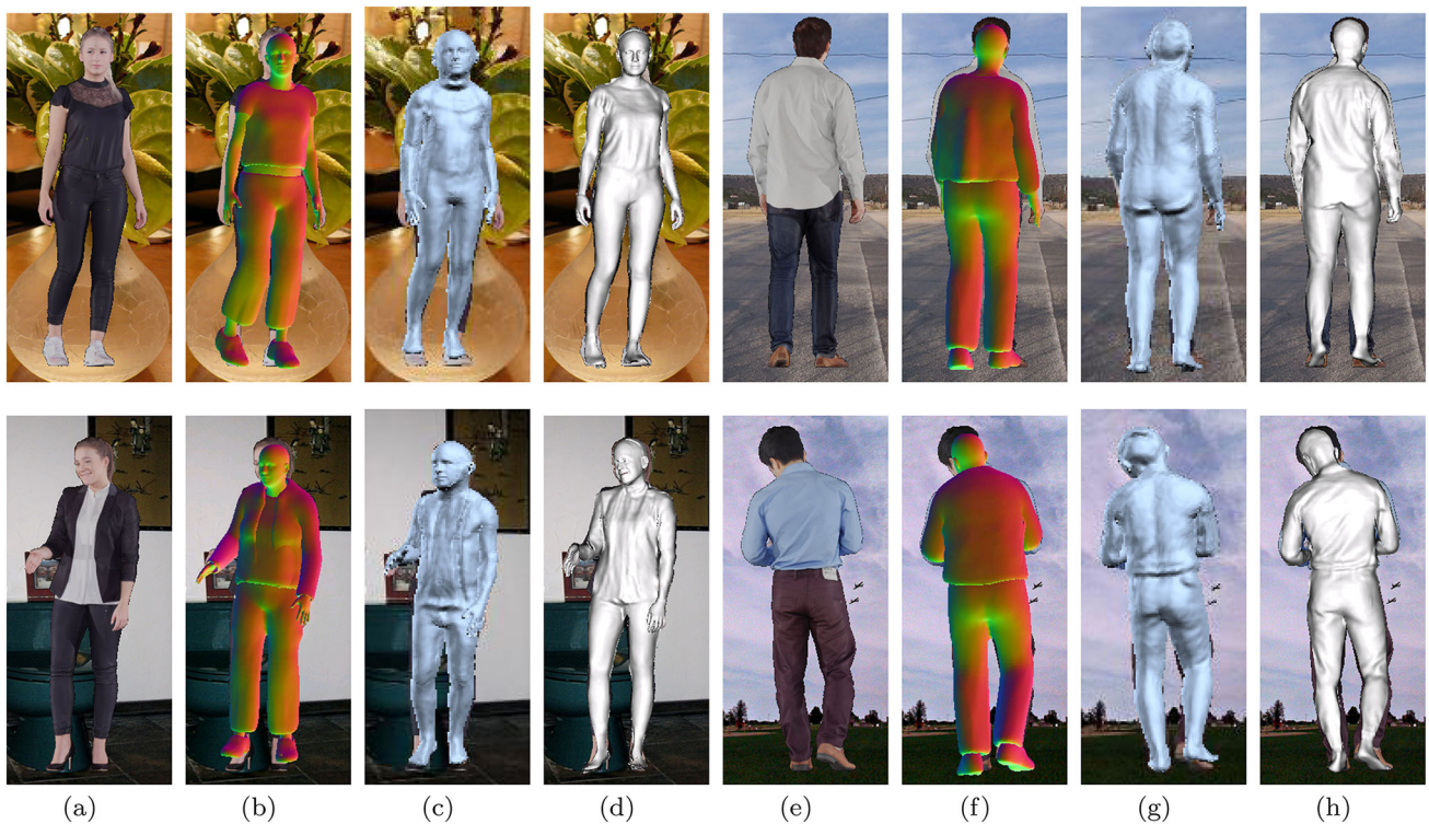
Fig. 6 Results on our collected dataset. We show the results of SMPLicit [27] (b, f), hmd [43] (c, g) and our implicit registration results (d, h) on the input image (a, e), respectively
