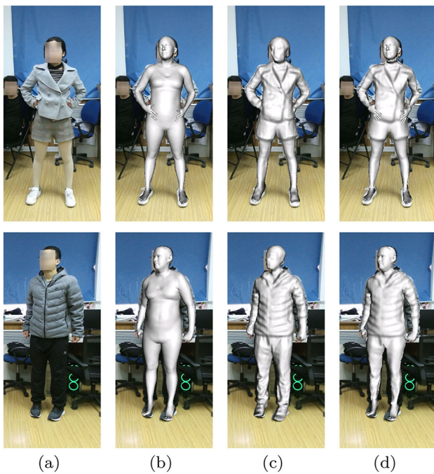
Fig. 3 Reconstruction results on DeepHuman dataset. We show the results of SMPL b , our implicit function results c and implicit registration results d on input image a , respectively
