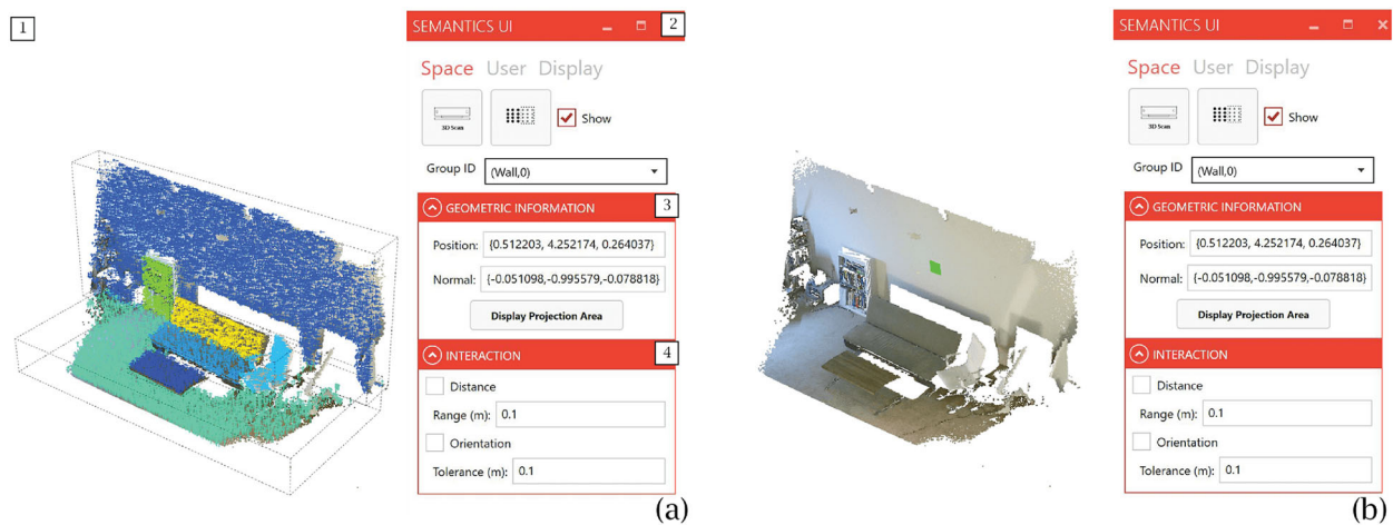
Fig. 5 Semantics Mapping UI (a) the visualization of 3D segmentation (1) the visual representation of the physical world and its semantic segmentation result (2) the control panel for scanning, segmenting, and annotating surfaces (3) the information panel for each segmented sur-
