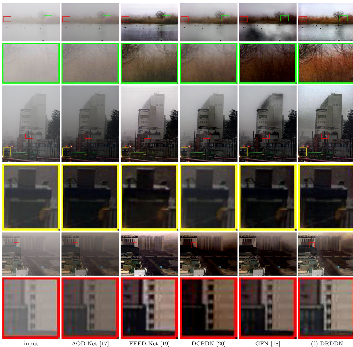
Fig. 8 The dehazing result of the proposed method and state-of-the-art methods on real-world dense hazy images. In the result of FEED-Net, there are artifacts shown in blue box. AOD-Net tends to leave haze in
