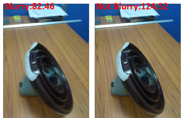
Fig. 3 Calculation of blurriness in the input images
